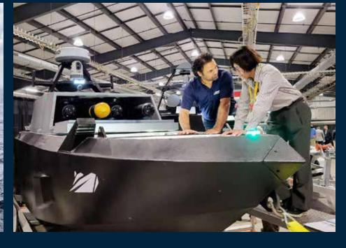
Introducing the Swift Sea-Stalker S3, an Unmanned Surface Vehicle (sUSV) designed for both remote and autonomous operations. Built with a durable aluminum hull and powered by a heavy-duty no. 2 diesel engine, the S3 offers high endurance and flexibility with two propulsion options: propeller and water-jet systems. Compliant with NATO STANAG 4586 and JAUS protocols, the S3 ensures seamless integration with joint operations.
