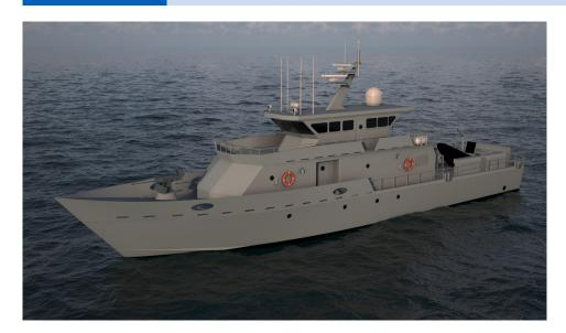
The 35 Meter Patrol Boat (Commercial Steel) has a steel hull and aluminum superstructure constructed of marine grade alloys.
